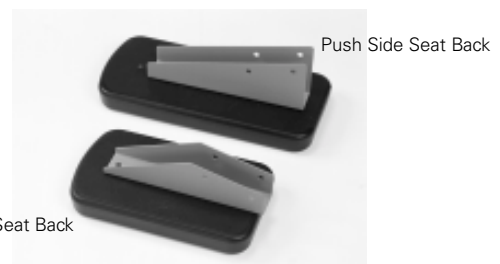
18. Assemble the Seat Backs to the Seat Back Brackets. Use two 3/8" by 7/8" screws for each Seat Back. Note that the more rounded end of the Seat Back is the top. The height of the seat back can be adjusted by the choice of mounting holes used. We suggest starting with the middle setting on the pull side, and the highest setting (lowest holes) on the push side. Reposition the seat backs according to the user's height if necessary.
