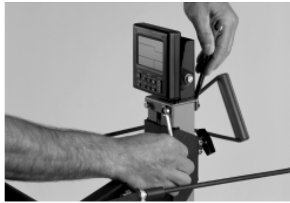
16b. Attach the Monitor Assembly to the top of the Mast using the two 1/4" by 2 1/2" screws and two 1/4" nuts. It doesn't matter which way you insert the bolts.
