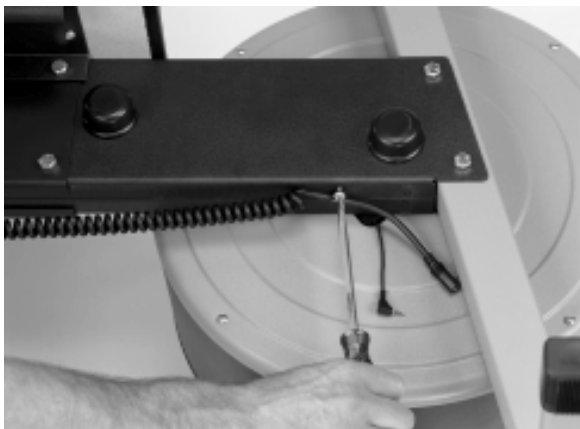
17b. Route the free end of the coiled cable through the fitting. Re-attach the Fitting to the Flywheel Assembly and connect the two plugs.
